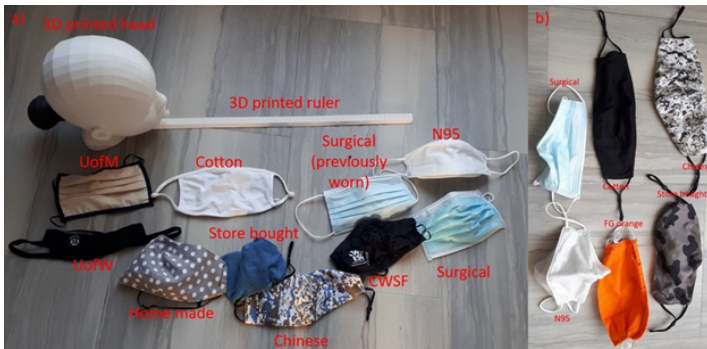
Figure 1. The materials for my experiment. Figure 1a): Experiments 1, 2, 3, and 4: The masks I tested in my project next to the 3D printed head used for testing and the 3D printed ruler used for measuring. The turkey baster is inside the head. Figure 1b) The masks I tested for Experiment 5. I used these new masks because the previous ones were covered in soil.
